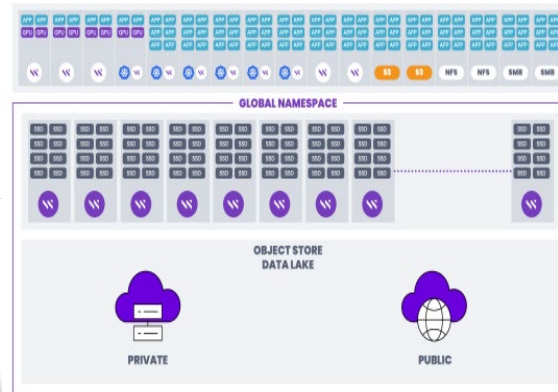
Figure 3: WekaFS combines NVMe flash with cloud object storage in a single global namespace
